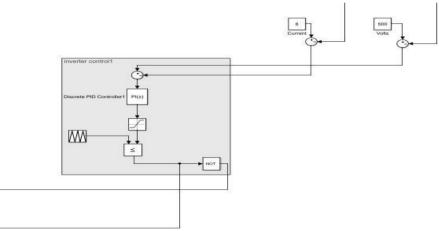
Figure 3: Voltage & Current Loop for the DCXs
