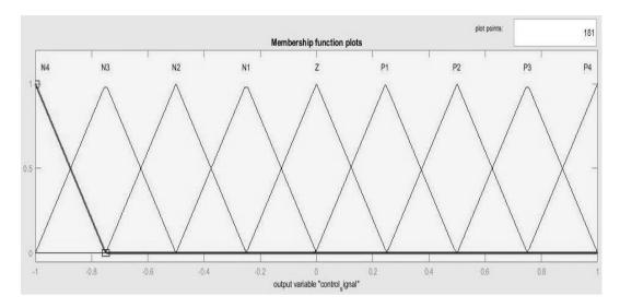
Figure 9: Control Signal Membership Function Plot
