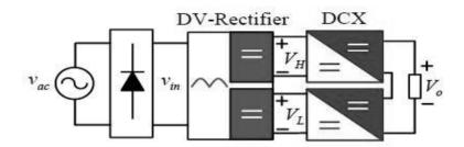
Figure 1: Dual Stage AC-DC Converter
