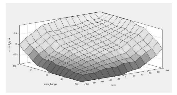
Figure 10: Control Surface Plot for Fuzzy Logic Controller
