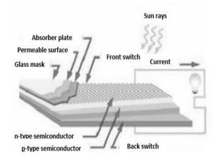
Figure 1: Structure of photovoltaic battery
