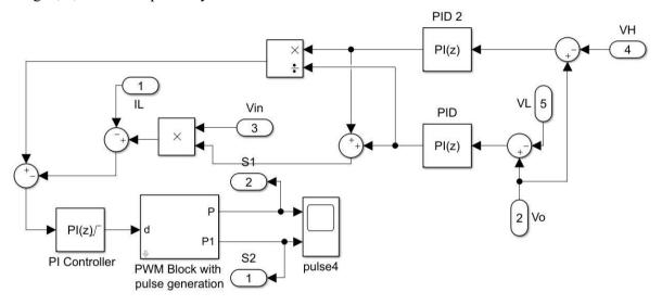
Figure 4: PWM Control Circuit for DV-Rectifier
