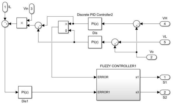
Figure 8: Fuzzy Logic Controller for DV-Rectifier
