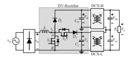
Figure 2: Proposed Dual Voltage Rectifier
